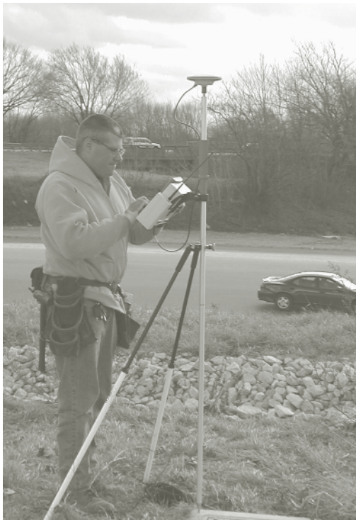
Ken Swift, McM Party Chief, setting up Leica SR530 receiver to obtain GPS location.
